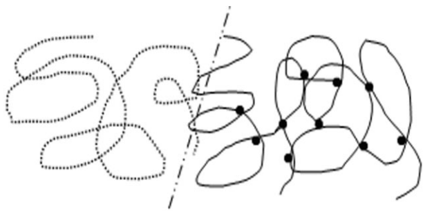
Scheme 1 An assuming pattern of molecular aggregation in noncovulcanized CIIR/PAC.
