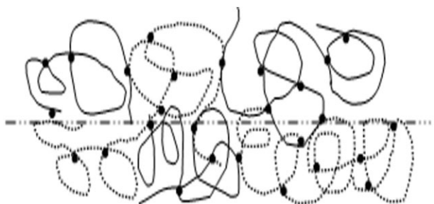
Scheme 2 An assuming pattern of molecular aggregation in covulcanized CIIR/c-PAC.
